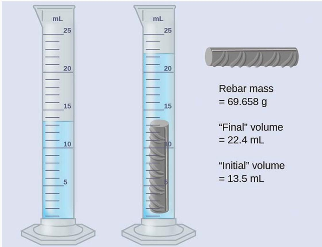
(a) Use these values to determine the density of this piece of rebar.
